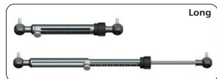
The inner tube is attached to a spring-loaded, black knurled adjustment knob (E). The adjustment knob mates with the threaded rod (F) in a manner such that the rod translates relative to the inner tube when the knob is rotated. This will provide gradual changes of overall strut length in 0.5-mm increments. A reference arrow with (+) sign located on the base of the adjustment knob (Fig. 4) indicates the direction of turning to perform strut elongation (distraction).
