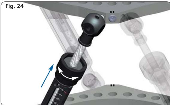
The gradual adjustment is achieved by pulling and rotating the adjustment knob (Fig. 24).
