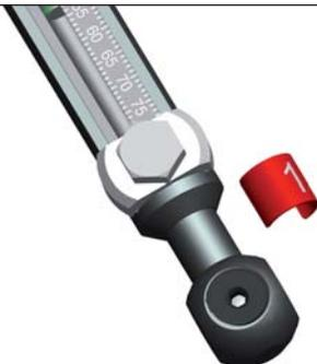
Snap the number clips into the groove at the tube end joint (Fig 16).
