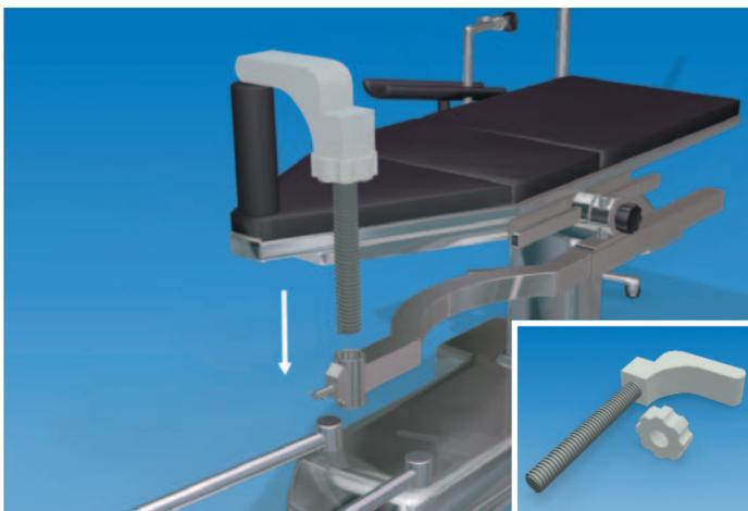
The Screw Jack of the Limb Support should be seated completely within the Housing of the Horizontal bar with the Nut turned so that it lies just beneath the Radiolucent Ledge.
